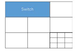
Using the grid layout can substantially reduce the time and effort required to draw parts on the screen, and increase the freedom of screen layout. With increased screen re-use, you can realize a reduction in overall HMI design time.
