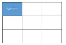
The size of rows and columns on the grid is relative to the resolution of the screen. If the screen resolution changes, the size of rows and columns adjusts accordingly. As a result, it is able to retain the location of parts relative to the original layout.
