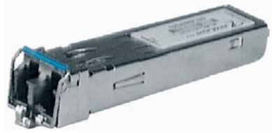
Figure 6: Fast Ethernet / Gigabit Ethernet fiber optic SFP module
