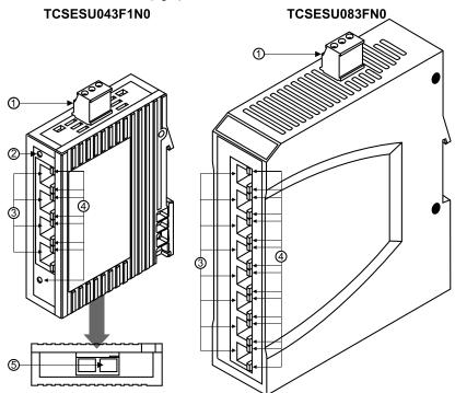
This illustration shows the 4-port TCSESU043F1N0 switch (left) and 8-port TCSESU083FN0 switch (right):
