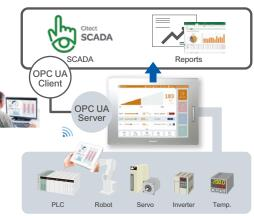
Connect to up to 10 drivers at the same time (PS6000/PS5000 and PC/AT and SP5000:10, GP4000\*/ST6000/STM6000:4, GP4100 Color Model:2)
