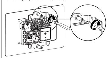
**NOTE:** If you exceed the recommended torque when tightening the installation fastener's screws, the front of this product may become distorted.
