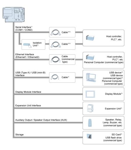
\*1 In order to use this as an isolation port, Isolation Unit is required. To use RS-232C isolation unit, set the #9 pin of the COM port to VCC.
