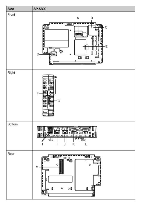
A: Auxiliary output/ Speaker output interface (AUX)
