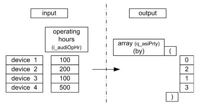
To activate this type of priority assignment, set the input parameter i\_ePrtyMode to the value Op.
