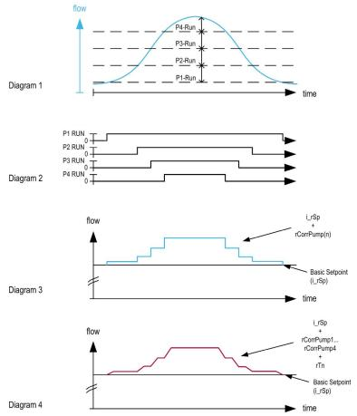
**Diagram 1:** The diagram shows the dependence of the total number of active pumps to the flow value and in dependence on the time.
