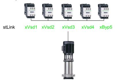
Example of using the stLink structured data type with fixed links (fixed link operational mode enabled):
