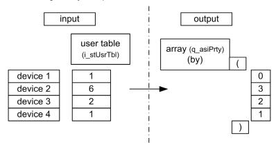
To activate this type of priority assignment, set the input parameter i\_ePrtyMode to the value User.
