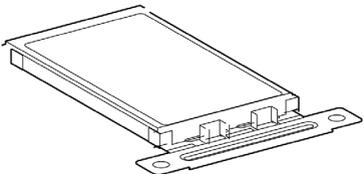
A perspective view of the same metal bracket as in step 4, but with a rectangular memory card inserted into the central cutout.                 |
