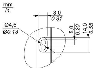
PE-B Atom N270 models are designed to be mounted using M4 screws:
