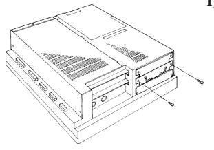
1) Unscrew the expansion slot's two (2) blank panel screws, and remove the blank panel.
