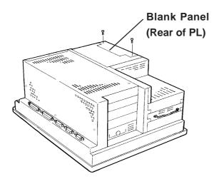
3) Unscrew the two attachment screws from the PL unit's rear face Blank Panel, and remove the cover.
