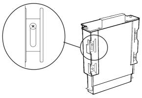
6) Insert the FDD unit so that its guide grooves fit the chassis guide ways. Push the unit in until its rear connector is connected securely.
