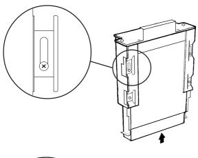
5) Slide the unit in the direction shown by the arrow, until the lower set screws' screw hole appears. Re-insert the two (2) lower set screws, and tighten both upper and lower (4) screws.
