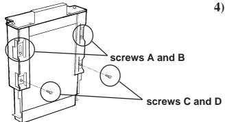
4) Loosen the PL-FD210 unit's two (2) upper adjustment screws (screws A and B), and remove the two (2) lower set screws (screws C and D).
