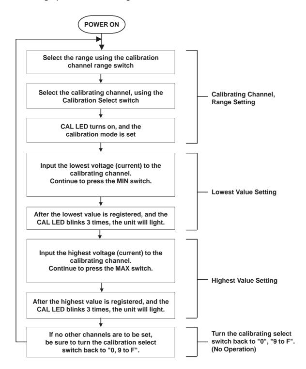
◆ 4 Channel Digital/Analog Conversion Unit (FN-DA04AH11) Analog Output Calibration Setting
