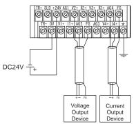
The left drawing explains the connection using ch1 and ch3 as – row. Each channel can be used connecting to voltage input units, or current input units.
