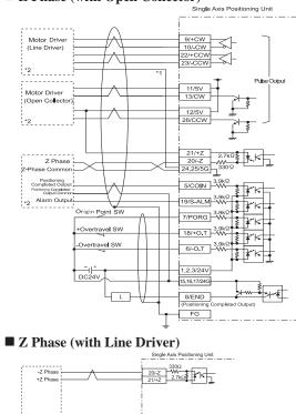
\*1 The FN-PC unit's live line is not isolated. If it is connected to a non isolated servo driver, be sure to connect the signal ground (5G) to prevent an over-current accident
