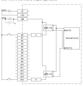
The I/O unit's power supply should be separated from Note: the sensor's power supply snound of the unit from being affected by external noise.
