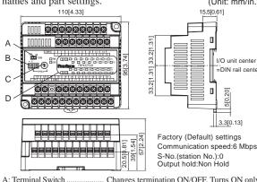
Changes termination ON/OFF, Turns ON only the unit connected at the end of the communica tion cable.
