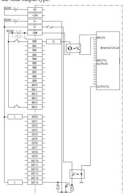
The I/O unit's power supply should be separated from the sensor's power supply to prevent the unit from being affected by external noise.
