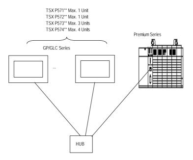
\* The maximum number of units indicated is when only GP units are connected. When other devices are connected via an ethernet connection, the number of GP units that can be connected is limited.
