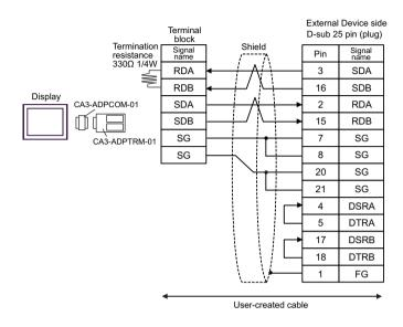
**NOTE** • As the External Device has the termination resistance built-in, you do not need to connect the termination resistance.
