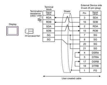
• As the External Device has the termination resistance built-in, you do not need to connect the termination resistance.
