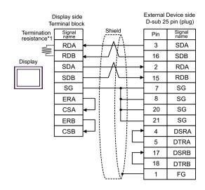
• As the External Device has the termination resistance built-in, you do not need to connect the termination resistance.
