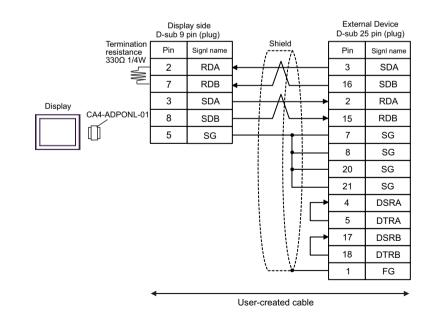
• As the External Device has the termination resistance built-in, you do not need to connect the termination resistance.
