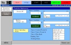
Displays grease-up, battery exchange time management, power on time
