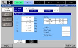
Displays the current value of Robot/Servo, tool info., system info.
