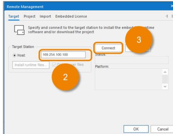
6. After confirming that the Remote Management tool connected to the Edge Box HMI and its status is displayed, click [Install Runtime Files].
