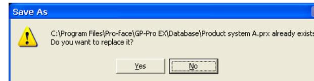
3. When receiving a project file that uses SD card/USB memory data such as Recipe Function (CSV data), the following dialog box will appear during the transfer. Please specify where to save the data. Click [OK] to return to the [Receive Project] dialog box and complete the transfer.
