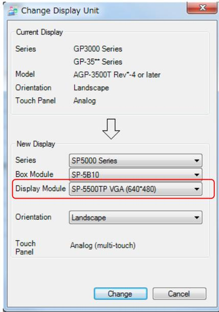
The Display Module can be Changed on the “Project” -> “System Settings” -> “Change Display Unit” screen of GP-Pro EX.
