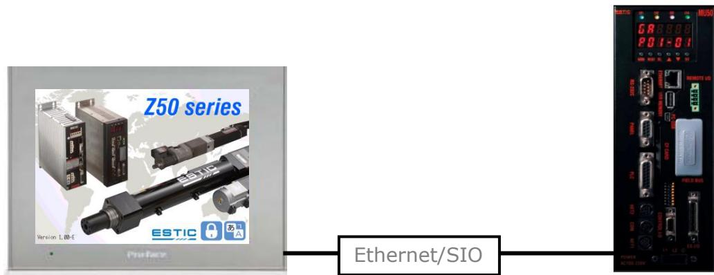
However, it is possible to connect multiple units with MU50. Please note that the indirect function is not used in this sample project file. If connecting with multiple units, peripheral connection settings and screen edits are required.
