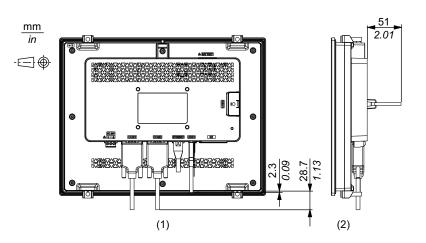
1 Rear 2 Right **NOTE:** All the above values are designed with cable bending in mind. The dimensions given here are representative values depending on the type of connection cable in use. Therefore, these values are intended for reference only.
