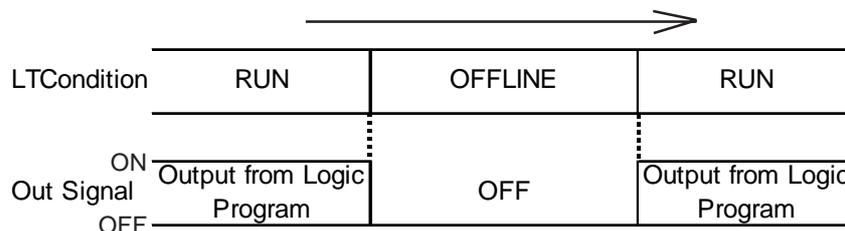
In order to initialize the LT or perform any self-diagnostics, you must change the LT to OFFLINE mode. The following explanation explains the two ways to enter this mode.
