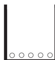
If different wires must be placed in the same duct, separate them with an earthed/grounded divider.
