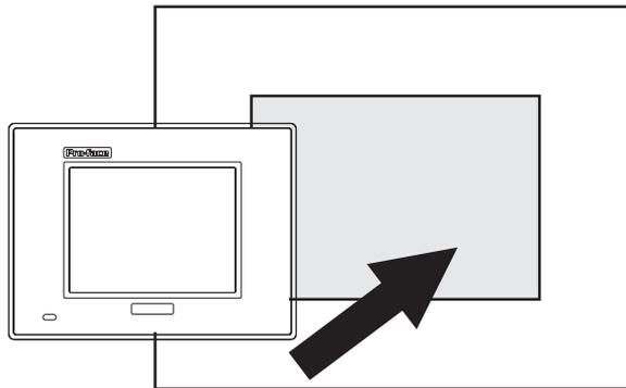
2. Insert the installation fasteners into the LT unit's insertion slots — two slots each, at the top and bottom of the unit (max. of 6, including sides).
