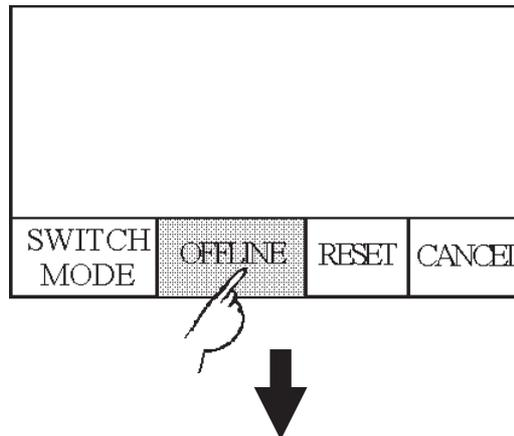
Entering OFFLINE mode will reset the LT unit's I/O. After confirming that this will not cause any problems, touch YES.
