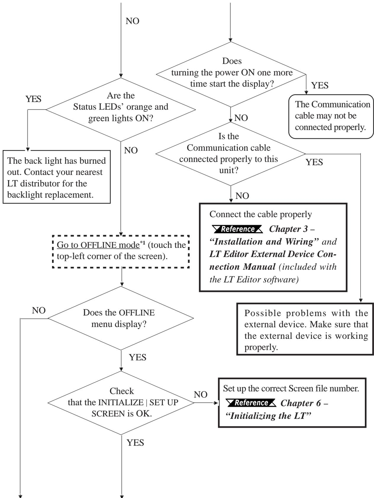
*1 To make the OFFLINE screen appear, turn the power OFF, then ON, and then touch the upper left corner of the screen within 10 seconds.*
