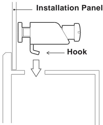
4. Be sure to pull the fastener back until it is flush with the rear of the attachment hole:
