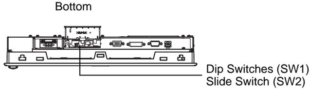
The factory default for the FP unit's Dip Switches and Slide Switch are as follows.
