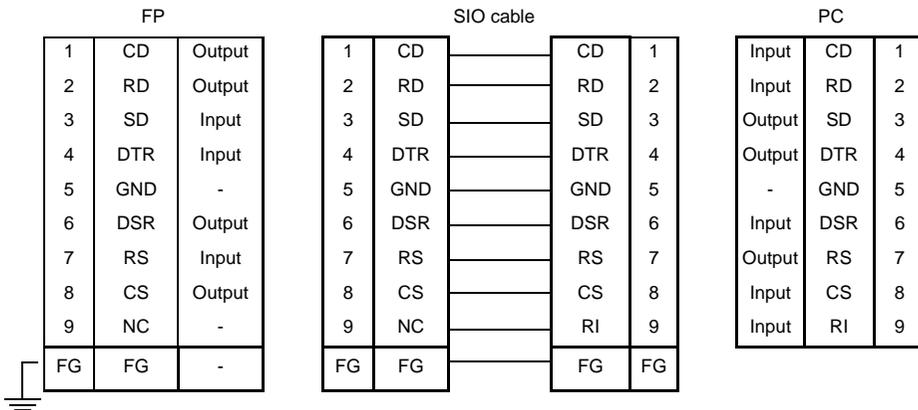
Signals and signal names used with the FP and the SIO cable (optional cable) are the same as those used for PCs. Also, the same pin is used on both sides of the optional cable so that you can connect the cable regardless of the cable direction.
