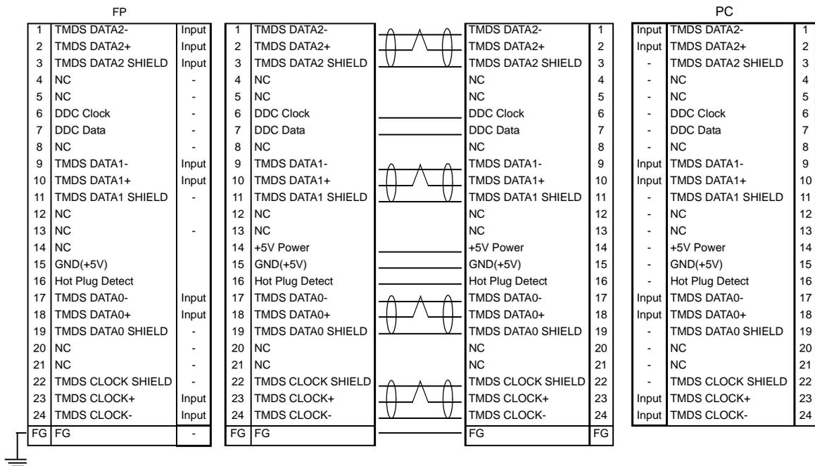
Signals and signal names used with the FP and the DVI-D cable (optional cable) are the same as those used for PCs. Also, the same pin is used on both sides of the optional cable so that you can connect the cable regardless of the cable direction.
