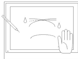
Do not use sharp or hard objects, such as a mechanical pencil or screwdriver, to push on the display. This could damage the unit.
