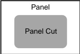
**NOTE** • Check that the installation panel or cabinet’s surface is flat, in good condition and has no jagged edges. Also, if desired, metal reinforcing strips can be attached to the inside of the panel, near the Panel Cut, to increase the panel’s strength.
