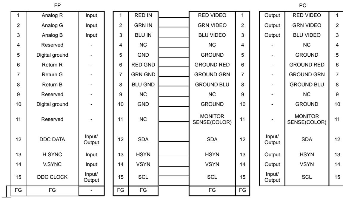
Signals and signal names used with the FP and the RGB cable (optional cable) are the same as those used for PCs. Also, the same pin is used on both sides of the optional cable so that you can connect the cable regardless of the cable direction.
