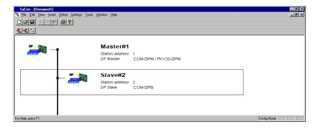
Right click on the COM-DPS and then select Slave Configuration, or (optionally) double click on the COM-DPS to bring up the Slave Configuration window.
