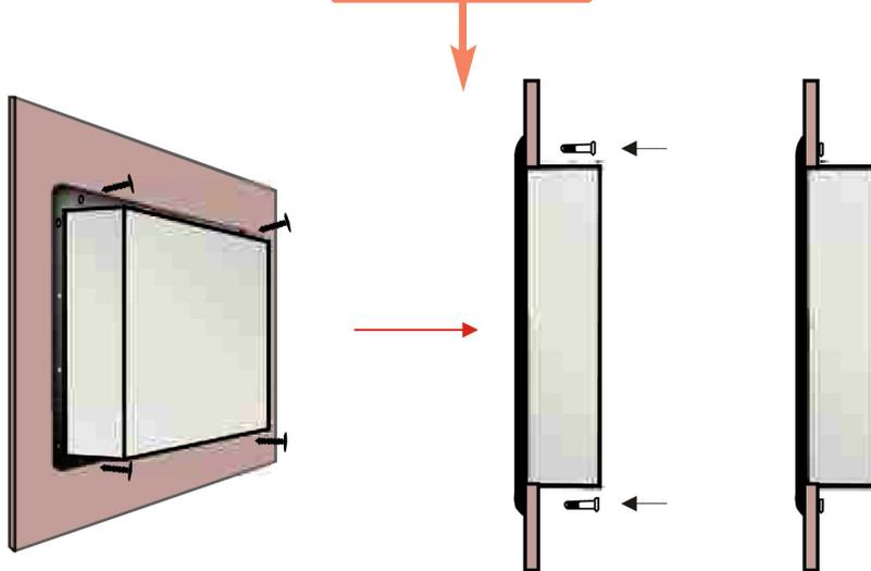
Use M3 screws to drill through the fixture into the mounting holes on the back side of IP65 front bezel
