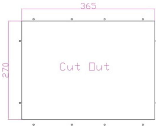
2. Screw from the back through the opening and mount the unit, make sure that the rubber in the right position to give IP protection
