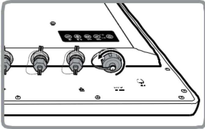
2. Plug the AC adapter to the DC-in jack of your device. Make sure the cable fits to the connector, then tighten the O-ring (by turning it clockwise) to secure the connection.
