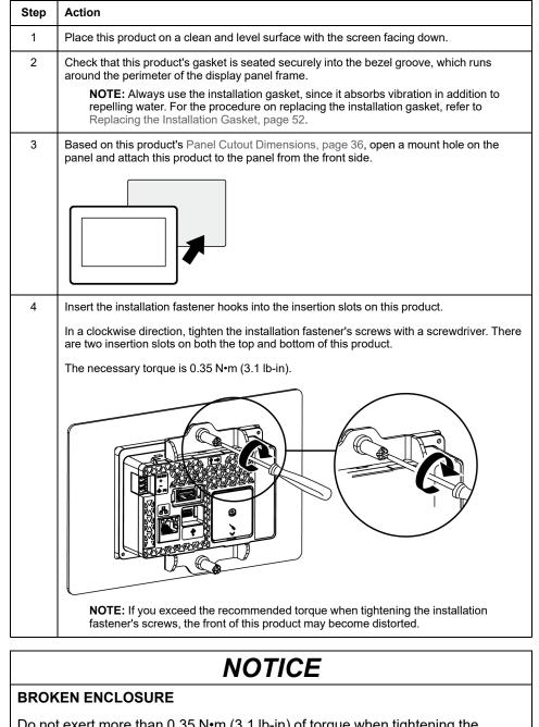
Do not exert more than 0.35 N·m (3.1 lb-in) of torque when tightening the fastener's screws.
