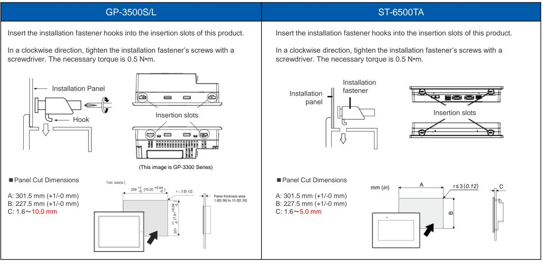
NOTE: The installation fasteners for GP3000 Series (P/N: CA3-ATFALL-01) cannot be used for ST-6500TA. Please use the fasteners for ST-6500TA (P/N: PFXZC3AT1). Please check <u>ST6000 Series Hardware Manual</u> for installation requirements and procedure.
