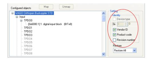
When connecting with WAGO 750-337, the Device type cannot be selected.
