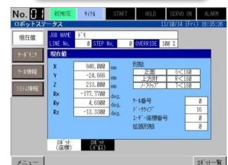
Display current value of Robot / Servo, Tool info. and System info
