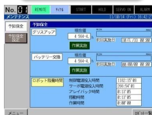
Manage Grease up, time for battery replacement and Display power on duration
